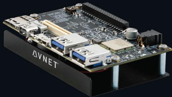
Ultra96™ is an Arm-based, Xilinx Zynq UltraScale+™ MPSoC development board based on the Linaro 96Boards specification.
