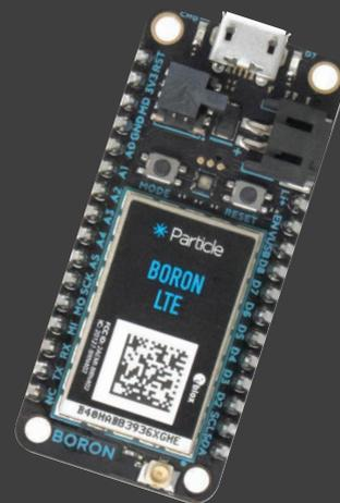
A powerful LTE CAT-M1/NB1 enabled development kit that can act as either a standalone cellular endpoint or LTE/3G/2G enabled gateway for Particle Mesh networks.
