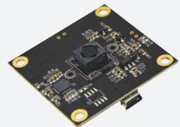
CAM8200-U is a 5-megapixel USB digital camera module designed by Embest Technology.
