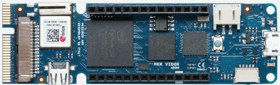
Arduino VIDOR 4000 is the first Arduino to feature an FPGA processor, all in the familiar MKR form factor.
