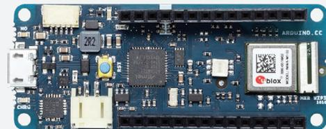
Arduino MKR WIFI 1010 is the evolution of the Arduino MKR1000 and is equipped with an ESP32 module made by U-BLOX.
