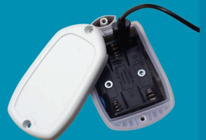
The Things Node is the perfect LoRa node to start prototyping your ideas without having to deal with bread boards, wires and sensors.
