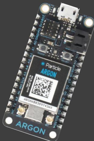
A Wi-Fi enabled development board that can act as either a standalone Wi-Fi endpoint or Wi-Fi enabled gateway for Particle Mesh networks.
